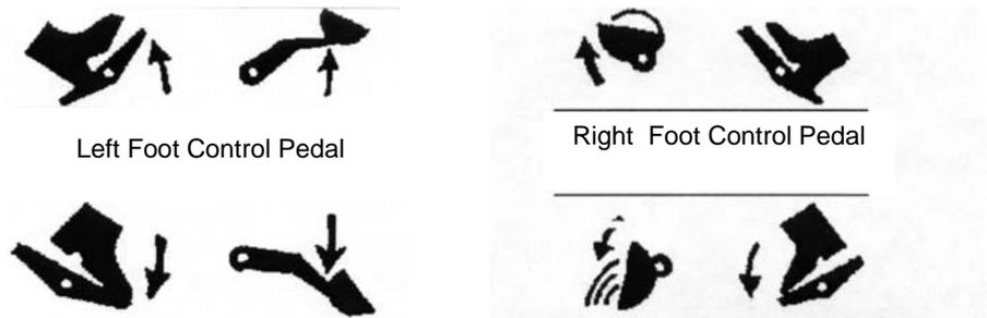
Figure 6.1.b. The hands and feet control the skid steer. Foot controls raise the lift arms (boom) and tilt or roll the bucket. The left heel raises the lift arms. The left toes lowers the lift arms. The right heel rolls the bucket back to load. The right toes tilt the bucket to dump the contents of the bucket. Practice these actions before proceeding to operate the skid steer.
