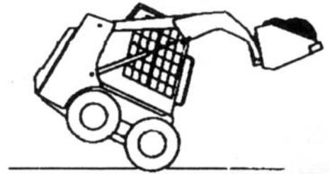
Figure 6.1.c. Skid steer loaders can tip forward if overloaded. This is an important reason to wear the seat belt, as well as understand the skid loader's load limitations.
