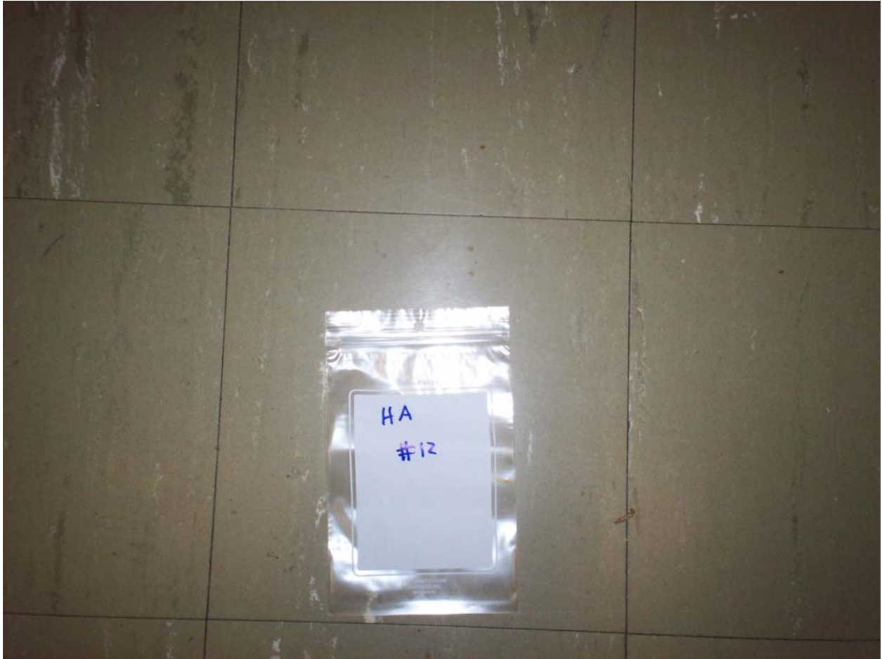
HA #12 – Asbestos containing 9” x 9” green floor tile with white streaks and associated non asbestos containing mastic
